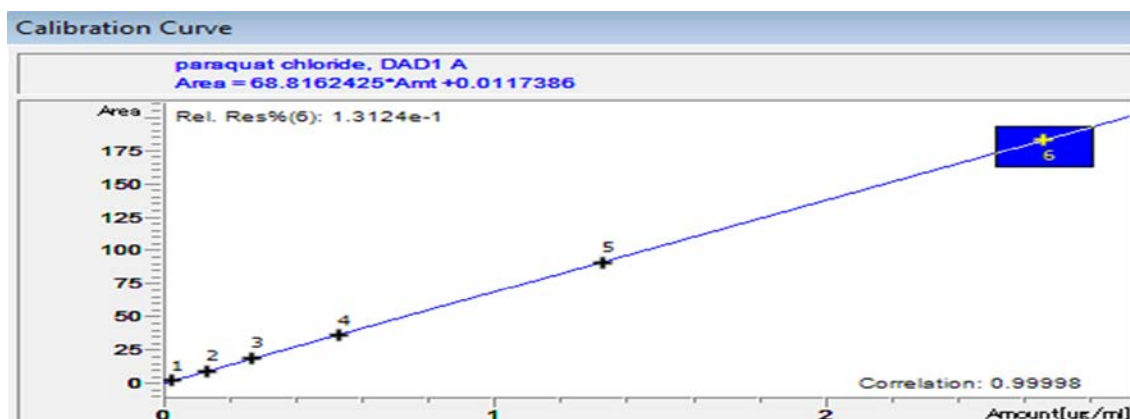
Figure 2 Calibration curve of paraquat standard solution 6 levels
