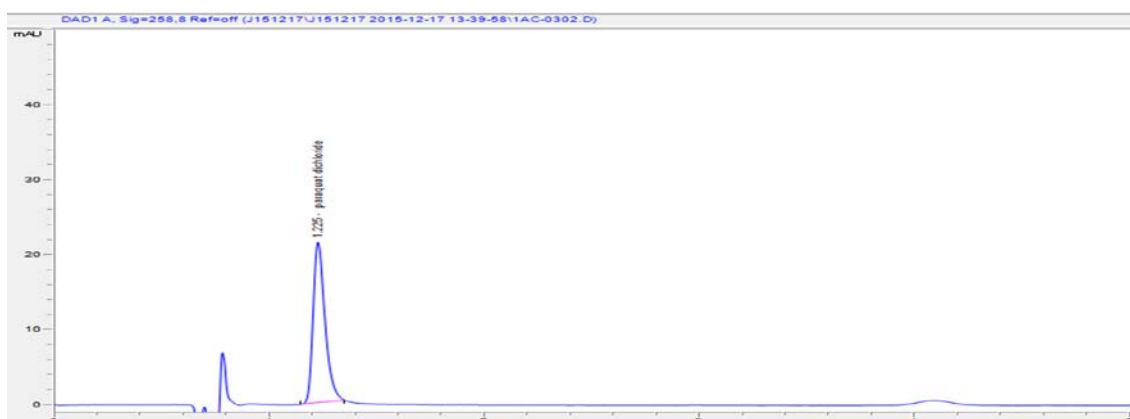
Figure 3 Chromatogram of paraquat standard solution ade by HPLC-DAD, concentration is 0.2656 µg/ml
