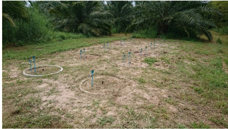
Figure 2 Installed soil moisture instrument (PR2) including with soil moisture measurement (Tensiometer)
