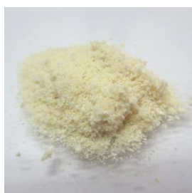
Figure 3 Carboxymethylcellulose (CMC) powder, which synthesized by reacting alkali-cellulose with chloroacetic acid, yield = 140.89%, purity = 95.33%, color score: L* = 84.122 a* = 1.11 and b* = 17.97
