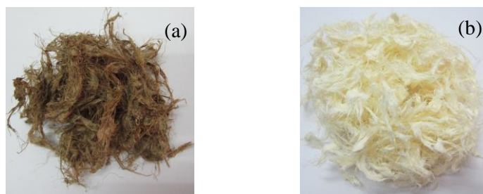
Figure 2 illustrates the cellulose from durian hulk. (a) Cellulose was extracted with 1 molar NaOH at 80-90°C for 1 hour. (b) Cellulose after bleaching with 30% H 2 O 2 at 80-90 °C for 20 min.
