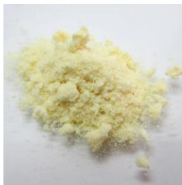
Figure 3 Carboxymethylcellulose (CMC) powder, which synthesized by reacting alkali-cellulose with chloroacetic acid, yield = 138.12%, purity = 95.63%, color score: L* = 85.82 a* = -0.67 and b* = 18.05
