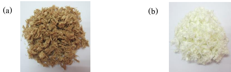
Figure 2 illustrates the cellulose from durian hulk. (a) Cellulose was extracted with 1 molar NaOH at 80-90 °C for 1 hour. (b) Cellulose after bleaching with 30% H 2 O 2 at 80-90 °C for 20 min.
