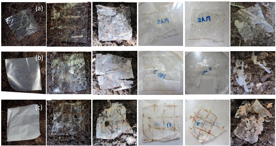
Figure 8 Apparent of PLA (a), PBS (b) and Mater-Bi ® (c) films during biodegradation studies in the soil burial test at \geq 30\% RH 29 \pm 1 °C pH 5 \pm 1 and 10,000 – 25,000 lux, at different stages of degradation (left to right: 0, 16, 42, 66, 100 and 161 days).
