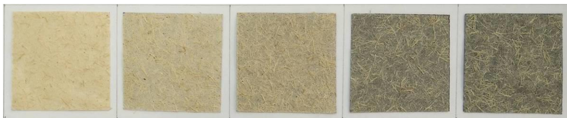
Figure 8 Ethylene absorber paper with various activated carbon powder content; left to right 0, 5, 15, 25 and 35% w/w
