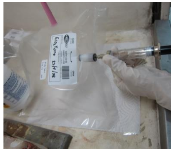
Figure 1 Tedlar bag was used for transferring ECO 2 FUME ® from cylinder to desiccator
