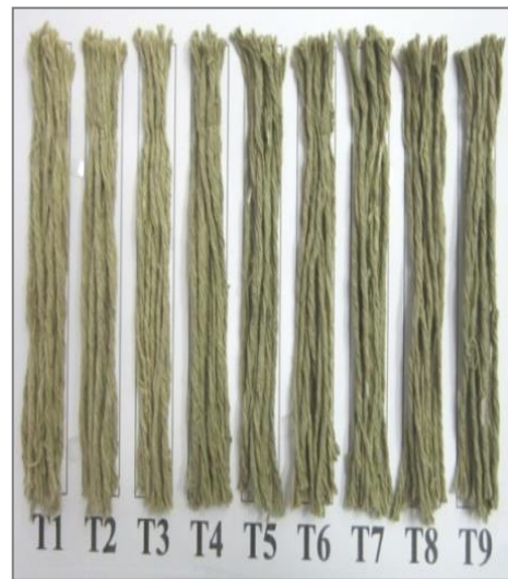
Figure 2 Effect of base solution on thread color changes (Left = Experiment 3, 12 months after storage ,T1= 100 °C water,T2= 0.25% NaOH ,T3= 0.25% Ca(OH) 2 ,T4= 5% lime water, and T5= dry cloth (control) : Right= Experiment 4, 9 months after storage , T1= 25°C water (control) , T2=30 min 100°C water,T3=50 min 100°C water, 30 min 0.25%Ca(OH) 2 ,T5= 50 min 0.25 Ca(OH) 2 , T6=30 min 5% lime water,T7= 50 min 5% lime water,T8= 30 min 20% ash water , and T9= 50 min 20% ash water)
