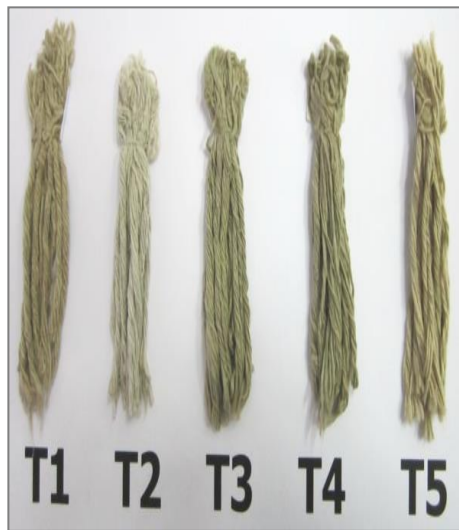
Figure 2 Effect of base solution on thread color changes (Left = Experiment 3, 12 months after storage ,T1= 100 °C water,T2= 0.25% NaOH ,T3= 0.25% Ca(OH) 2 ,T4= 5% lime water, and T5= dry cloth (control) : Right= Experiment 4, 9 months after storage , T1= 25°C water (control) , T2=30 min 100°C water,T3=50 min 100°C water, 30 min 0.25%Ca(OH) 2 ,T5= 50 min 0.25 Ca(OH) 2 , T6=30 min 5% lime water,T7= 50 min 5% lime water,T8= 30 min 20% ash water , and T9= 50 min 20% ash water)
