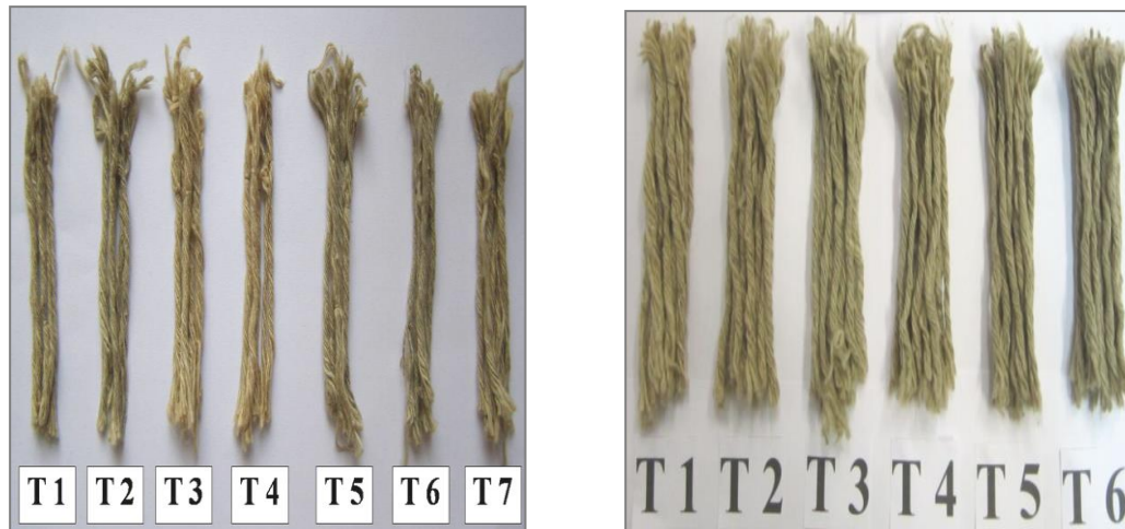
Figure 1 Effect of heat, acid, base and salt solution on thread color changes (Left = Experiment 1, 3 months after storage, T1 = 25°C water (control) ,T2 = 50 °C water, T3 = 1% citric acid pH 2, T4 = 1% citric acid pH 5, T5= 0.25% NaOH pH 8, T6=0.25% NaOH pH 11, and T7= 1% NaCl : Right = Experiment 2, 12 months after storage T1=25°C water (control), T2=50°C water, T3=0.25% NaOH, T4= 1% NaOH, T5=0.25% Ca(OH) 2 , and T6= 1% Ca(OH) 2
