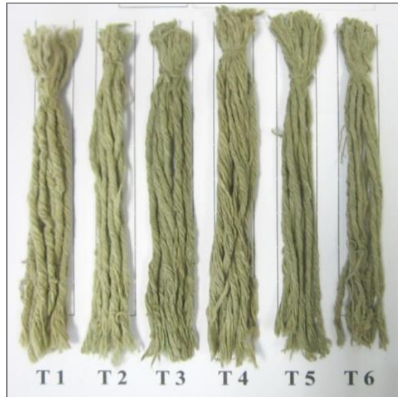
Figure 4 Effect of base solution on thread color changes at 1 month after storage T1=25°C water (control), T2= 100 °C water , T3= 0.25% Ca(OH) 2 , T4= 5% lime water, T5= 5% ash water, และ T6= 20 % ash water)
