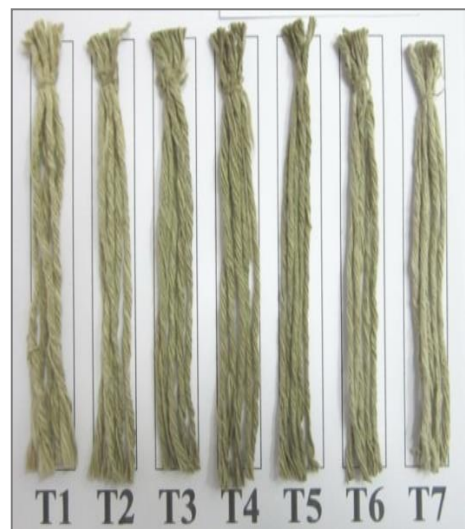
Figure 3 Effect of base solution on thread color changes of experiment 5 at 4 months after storage (Left= kept in the dark: Right kept in the light) T1=25°C water (control),T2=
