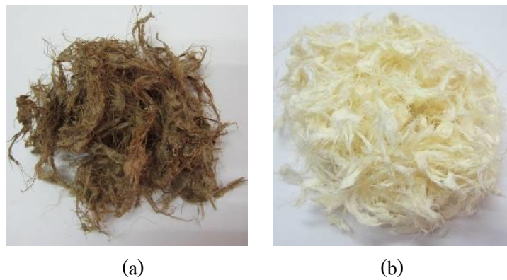
Figure 7 Illustrates the cellulose from banana pseudo-stem. (a) Cellulose was extracted with 1 molar NaOH at 80-90 °C for 1 hour and (b) cellulose after bleaching with 30% H 2 O 2 at 80-90 °C for 20 min.
