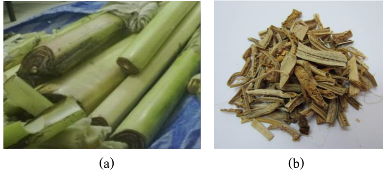
Figure 5 Illustrates the banana pseudo-stem (a) and after dried at 55 °C (b)
