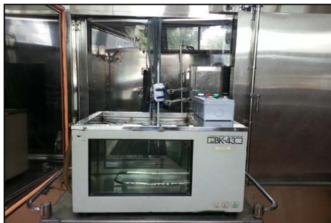
Figure 10. Calibration sensor of resistance thermometers.
