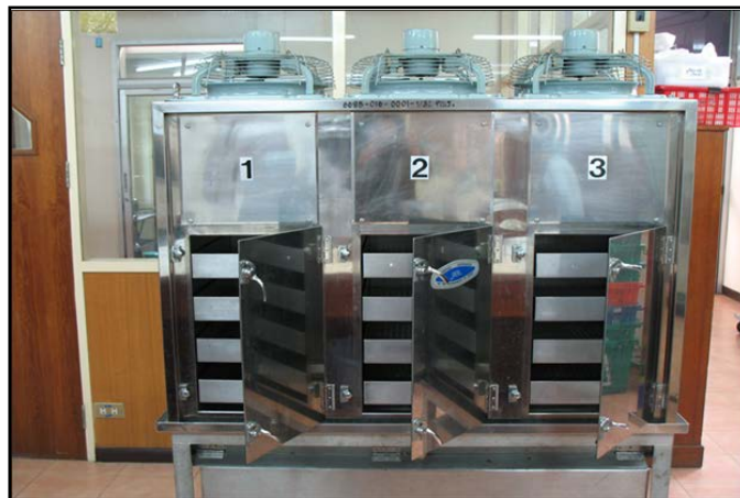
Figure 16. Showing cooling system (differential pressure type) model: SHS-12.
