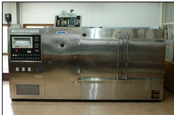
Figure 8. Sanshu vapor heat treatment system (differential pressure type) model: EHK-1000D.
