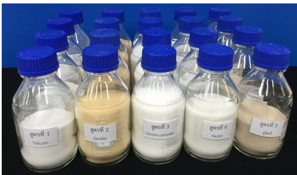
Figure 2 wettable powder bioproducts with talcum, zeolite, calcium carbonate, kaolin and phumai sulfate carriers, respectively
