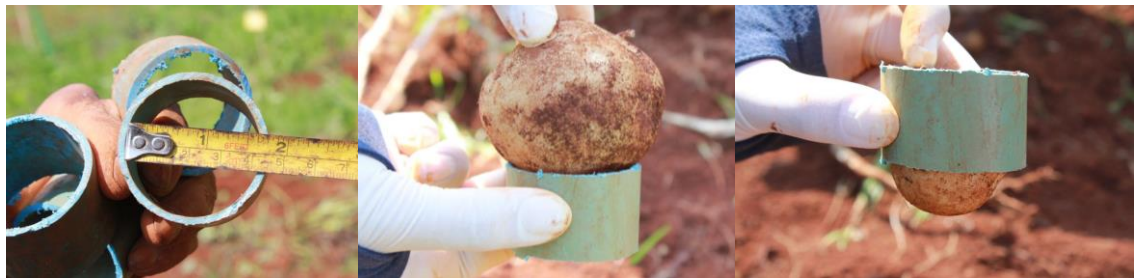
Figure 5 The equipment used to measure the tuber size of the potato for factory supply
