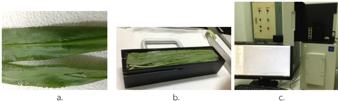
Figure 1 a. the vegetable leaves with whiteflies b. cell placing vegetable sample for measuring light absorption in NIR spectrometer c. the NIR spectrometer
