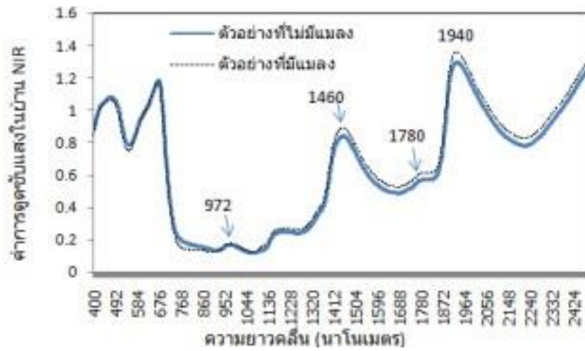
Figure 2. The NIR absorbance of vegetables with and without whitefly at different wavelengths by NIR spectrometer
