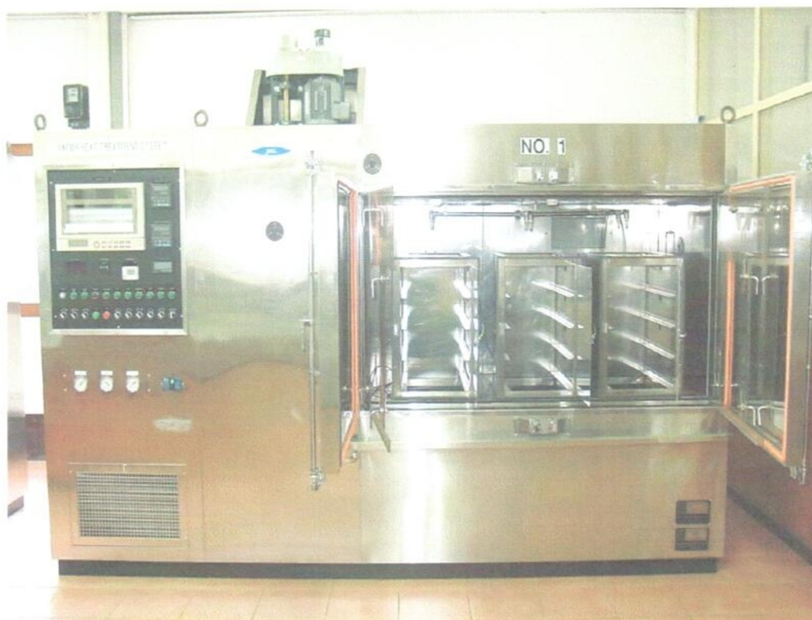
Figure 7 Sanshu' Vapor Heat Treatment System (Differential Pressure Type model EHK-1000 D)
