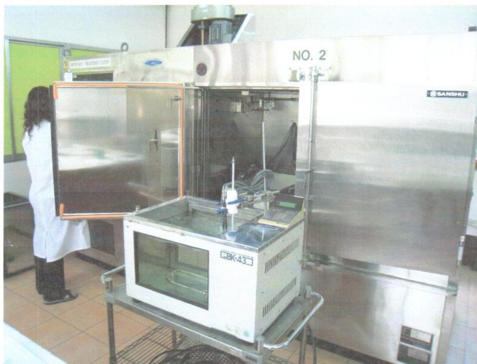
Figure 7 Sanshu' Vapor Heat Treatment System (Differential Pressure Type model EHK-1000 D)
