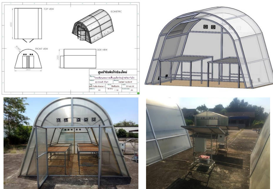
Fig.3 Green solar drying plant parabolic shape
