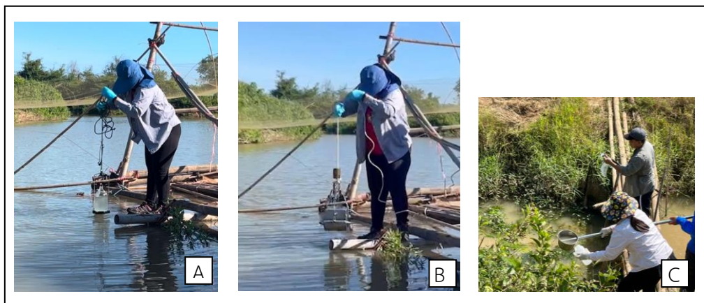
Figure 2 Water and sediment sampling : (A) by water sampler (B) by grab sampler and (C) by water ladle
