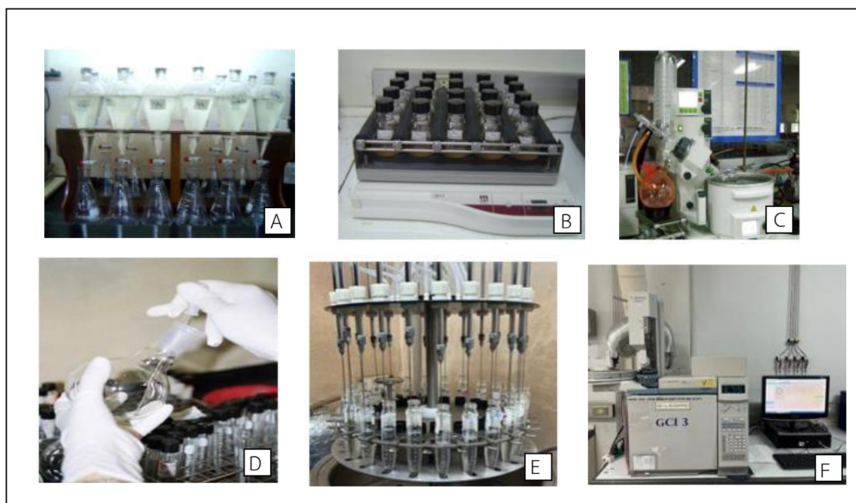
Figure 3 Steps of pesticide residues extraction and analysis : (A) water extraction by Liquid – liquid extraction (B) sediment extraction by solid – liquid extraction (C) concentrated by rotary evaporator (D) rinse the concentrated sample with solvent (PR grade) (E) concentrated by Nitrogen evaporator and (D) analyzed the pesticide residues by Gas Chromatograph (GC)
