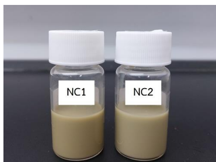
Figure 3 Encapsulated neem extract product in capsule suspension form (CS); NC1 by 0.5% PLLA and NC2 by 4% PLLA
