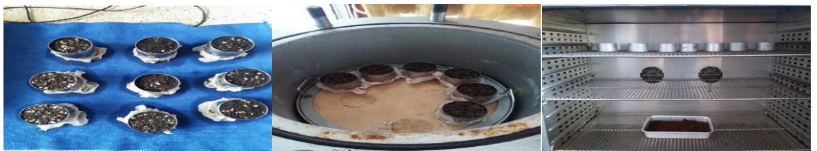
Figure 3 After growing media were pressured in 15 atmospheres for permanent wilting point (PWP) until water drainage finished to weighing following with samples were dried at 60°C for 3 days.
