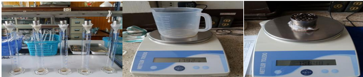
Figure 2 Growing media water was drained until finished for filed capacity condition (FC) after that on both water drained amount and material samples to weighting.
