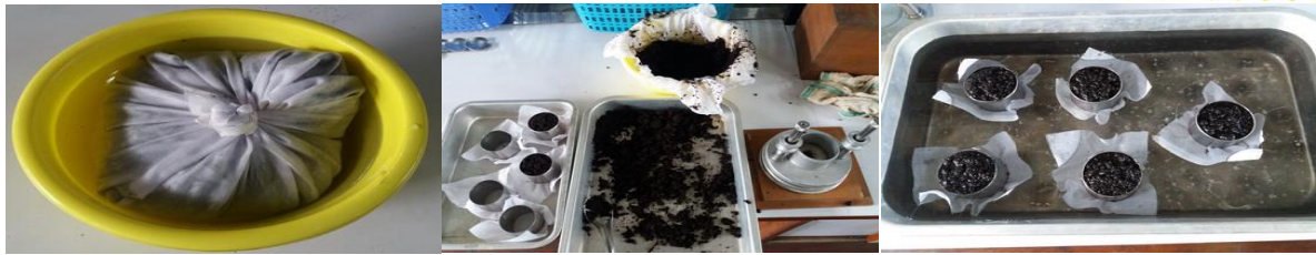
Figure 1 Materials were compacted with cores by gravimetric method after that saturated with water for 1 hour.
