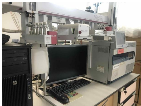
Figure 4 Gas Chromatograph-Tandem Mass Spectrometer received from the Department of Agriculture in 2016.
