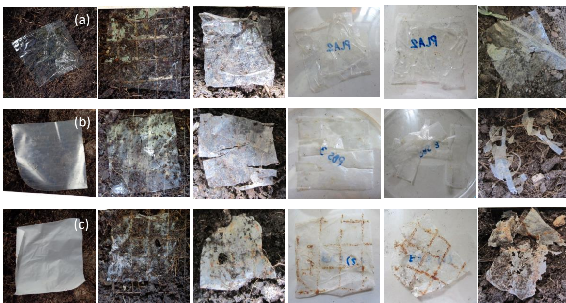
Figure 8 Apparent of PLA (a), PBS (b) and Mater-Bi ® (c) films during biodegradation studies in the soil burial test at \geq 30\% RH 29 \pm 1 °C pH 5 \pm 1 and 10,000 – 25,000 lux, at different stages of degradation (left to right: 0, 16, 42, 66, 100 and 161 days).
