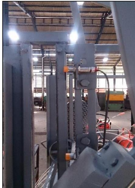
รูปที่ 17 Proximity sensor is set up at the moving path of the DC motor.
