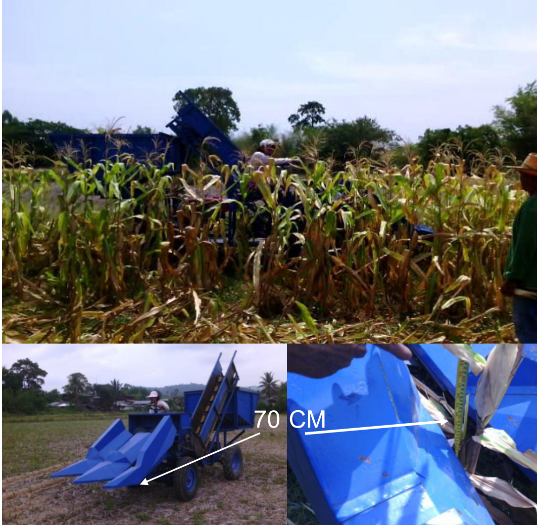
Fig.3 Level head Maize snapper for work
