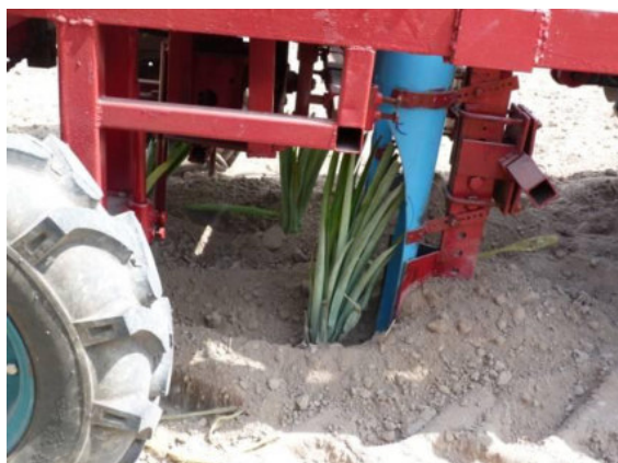
Figure 13 Characteristics and down out pineapples suckers through the tube
