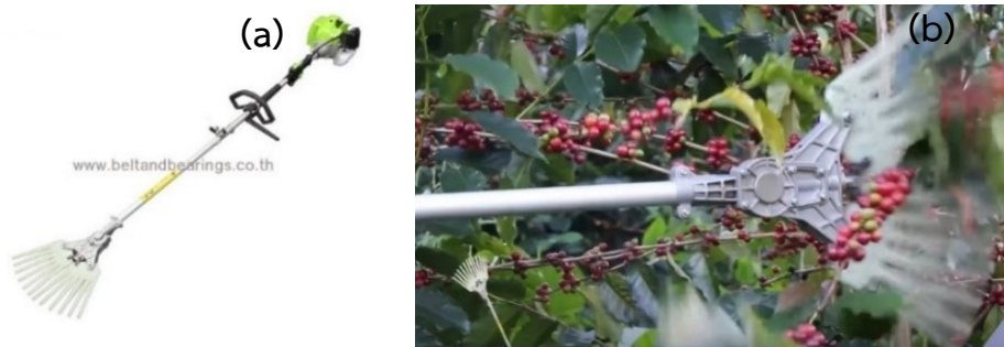
Figure 3 Chinese coffee harvester (a) and harvesting coffee by chinese harvester (b).
