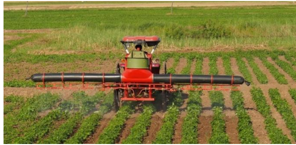
Figure 8 Air assist boom sprayer working in mung bean field
