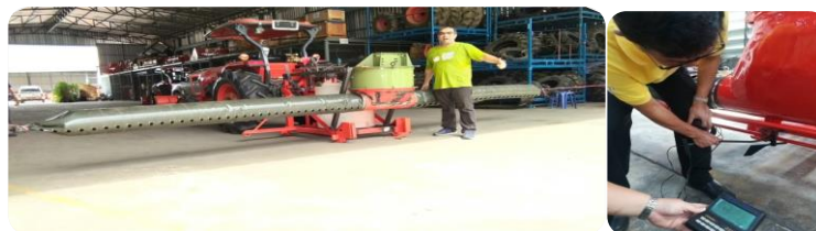
Figure 4 Air flow measurement test in laboratory
