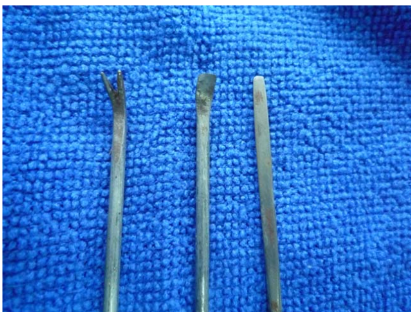
The flat end of the wire into the V (V) and the flat look.
