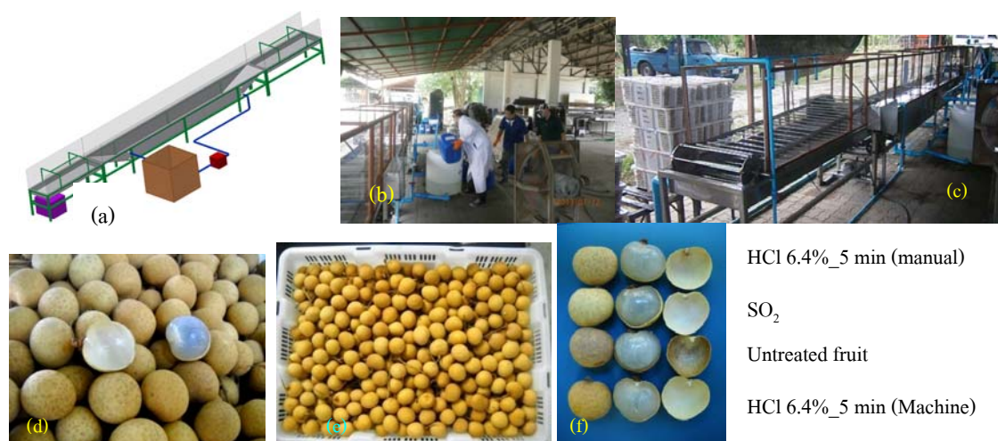
Figure 3. Model of original HCl dipping machine (a) and 10 meters in length, (b) staff demonstrated carefully during pouring HCl into plastic container, protected him with glove in hand, covered nose with mask and using lectric fan help (c) and HCl dipping machine made by stainless steel (d). Fruit appearance after dipped HCl 6.4% for 5 min before transportation (a) and arrived at Singapore (b) and compared between 4 treatments at 1 st day during storage at 5°C for 20 days.
