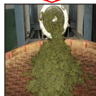
Rolled for crumbing by Cutting machine (modified meat grinder)
