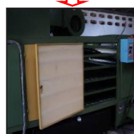
Dried at 110°C by Dryer machine until tea moisture lower than 13%
