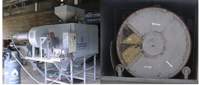
Figure 4. Rotary Dryer capacity 280 kgs
