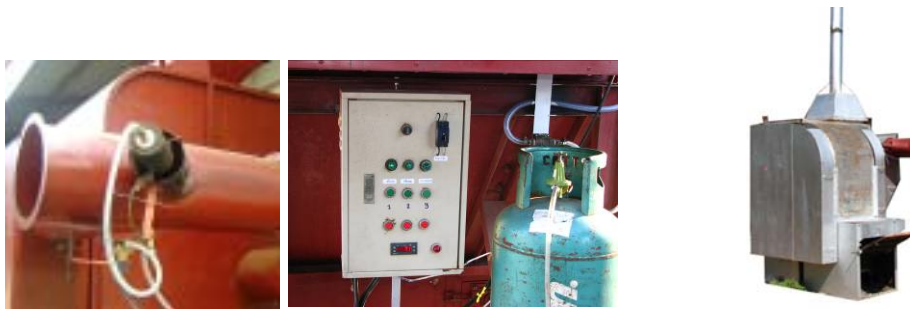
Figure 13. Gas burner together with temperature controller and heat exchanger of biomass furnace
