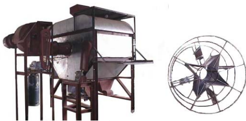
Figure 5. Rotary Dryer capacity 800 kgs
