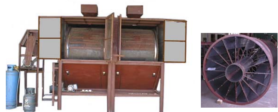
Figure 6. Rotary Dryer capacity 1,500 kgs
