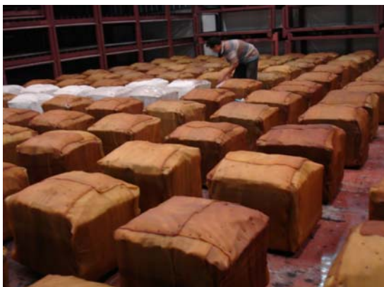
Figure 5. coating with glue rubber powder solution
