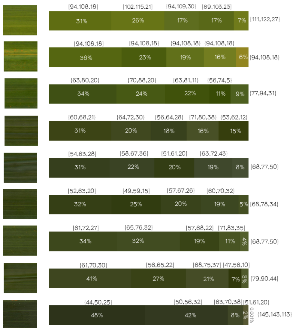
Figure 3 Color value from color grouping of nitrogen levels in oil palm leaf.
