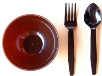
Figure 10 Packaging made from injection-molded plastic mixed with P3 formula
