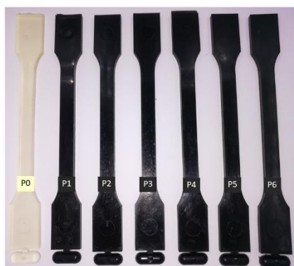
Figure 6 Visual appearance of the injection-molded pieces of polylactide (PLA)/extracted spent coffee grounds (ESCG): (P0) neat PLA; (P1) PLA+3%ESCG; (P2) PLA+5%ESCG; (P3) PLA+7%ESCG; (P4) PLA+9%ESCG; (P5) PLA+11%ESCG; (P6) PLA+13%ESCG
