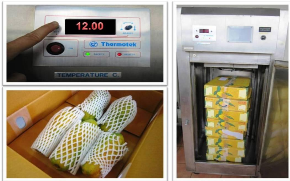
Fig. 4 After treatment : The heat-treated and untreated fruits were kept in constant temperature and humidity chamber at 12^{\circ}\text{C}\pm 1 and 75\pm 5\% RH. For evaluate the quality of fruits 7 days after treatment.
