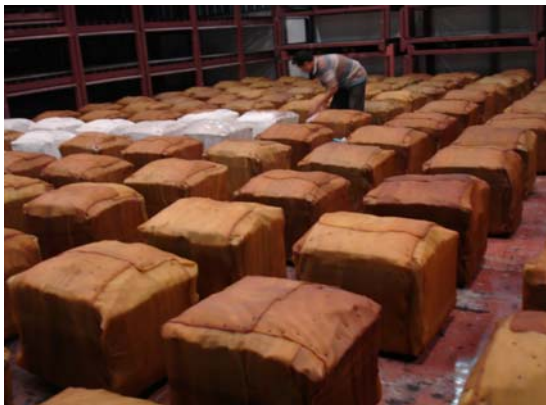
Figure 5. coating with glue rubber powder solution
