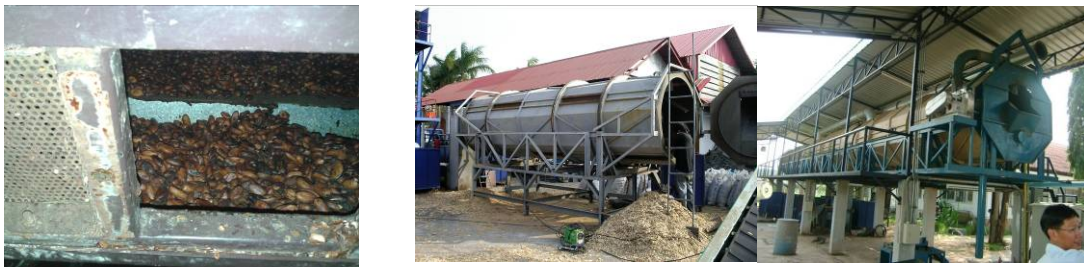
Figure 19. Drying test of cocoa Figure 20. Using of large scale rotary dryer for biomass drying
