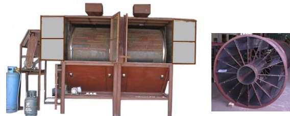
Figure 6. Rotary Dryer capacity 1,500 kgs
