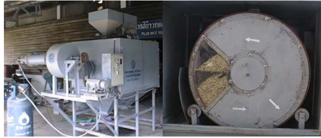
Figure 4. Rotary Dryer capacity 280 kgs
