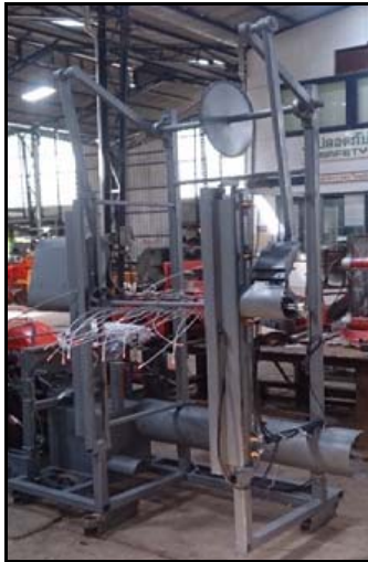
Figure 10 The primary sugarcane leaf pruning mechanism.
