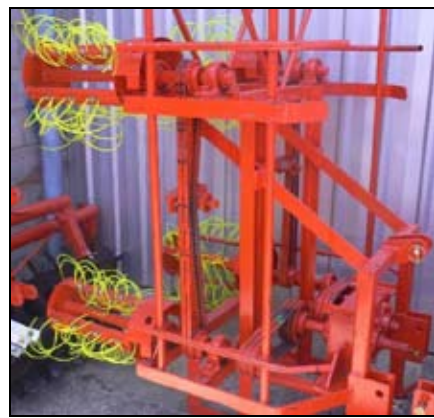
Figure 2 General Sugarcane Leaf Pruning Machine used in the present.
