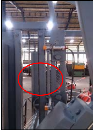
Figure 12 Proximity sensor's set up at the moving path of the DC motor.
